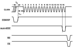
Figure 5. Using an External Clock
