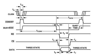
Figure 7. Conversion Sequence Timing Diagram (BUSY Mode)
