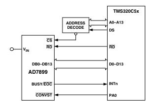
Figure 15. AD7899–TMS320C5x Interface
