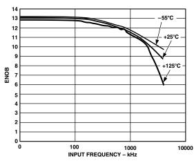
Figure 11. Effective Numbers of Bits vs. Frequency
