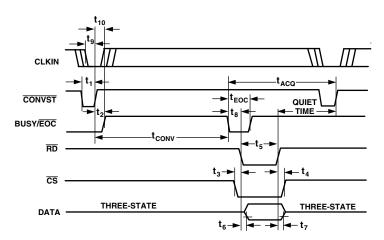
Figure 6. Conversion Sequence Timing Diagram (EOC Mode)
