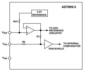
Figure 4. AD7899-3 Analog Input Structure
