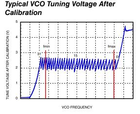
[1] Fractional Mode, 50 MHz Crystal, R=1, ~80 kHz Loop BW, (Loop filter values: Contact factory for component values) 2mA Charge Pump, -385µA Offset.
