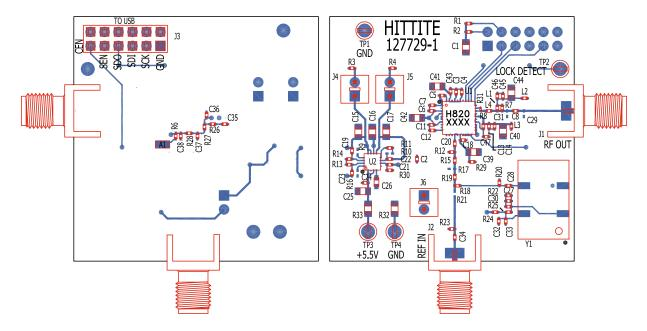
The circuit board used in the application should use RF circuit design techniques. Signal lines should have 50 Ohm impedance while the package ground leads and exposed paddle should be connected directly to the ground plane similar to that shown. A sufficient number of via holes should be used to connect the top and bottom ground planes. The evaluation circuit board shown is available from Hittite upon request.
