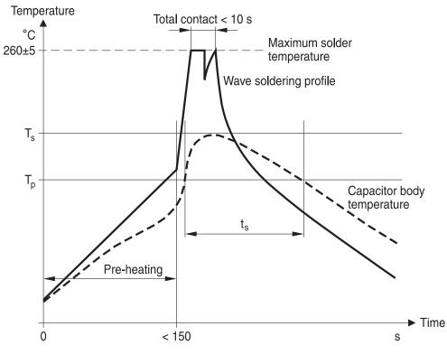
$\label{eq:Ts} T_{s}: \mbox{Capacitor body maximum temperature at wave soldering} \\ T_{p}: \mbox{Capacitor body maximum temperature at pre-heating} \\ \mbox{KMK1745-A-E} \\ \mbox{KMK175-A-E} \\ \mbox{KMK175-A-E} \\ \mbox{KMK175-A-E} \\ \mbox{KM$
