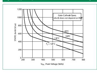
Figure 10. Typical Exponential Static dv/dt Vs Junction Temperature
