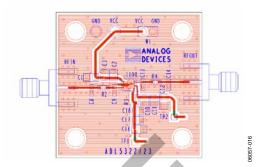
Figure 17. Evaluation Board Component Side View
