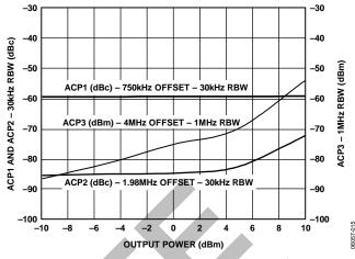
Figure 16. CDMA2000 ACP vs. Output Power per Carrier; 4 Adjacent Carriers
