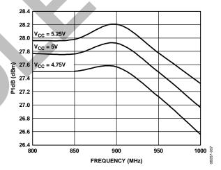
Figure 7. P1 dB vs. Frequency,  $V_{CC}$  = 4.75 V, 5 V, and 5.25 V,  $T_A$  = 25°C
