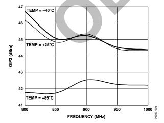
Figure 5. OIP3 vs. Frequency,  $V_{CC} = 5 \text{ V}$ ,  $T_A = -40 ^{\circ}\text{C}$ ,  $+25 ^{\circ}\text{C}$ , and  $+85 ^{\circ}\text{C}$
