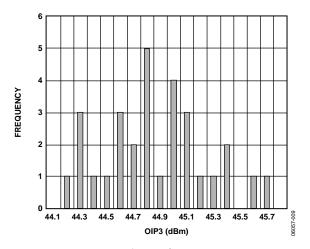
Figure 9. Distribution of OIP3 at 850 MHz
