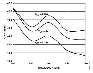
Figure 8. OIP3 vs. Frequency,  $V_{CC}$  = 4. 75 V, 5 V, and 5.25 V,  $T_A$  = 25°C
