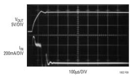
Figure 8. Input Current at Start-Up Without Soft-Start
