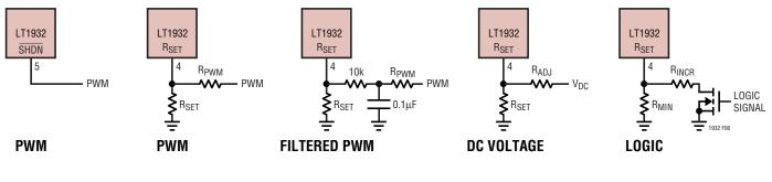
Figure 6. Five Methods of LED Dimming
