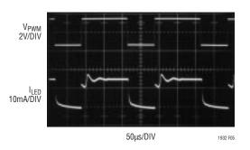
Figure 5. PWM Dimming Using the SHDN Pin
