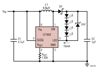
Figure 4. LED Driver with Open-Circuit Protection
