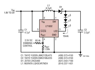
2-Cell Driver for Three White LEDs
