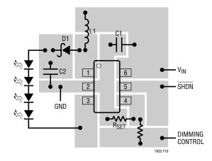
Figure 10. Recommended Component Placement
