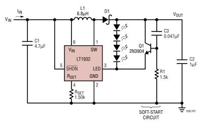
Figure 7. Soft-Start Circuit for the LT1932
