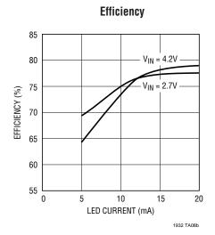
Li-Ion Driver for Three White LEDs
