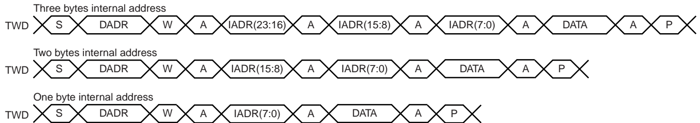
Figure 29-10. Master Write with One, Two or Three Bytes Internal Address and One Data Byte
