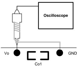
Figure 5. Voltage Ripple Measurements
