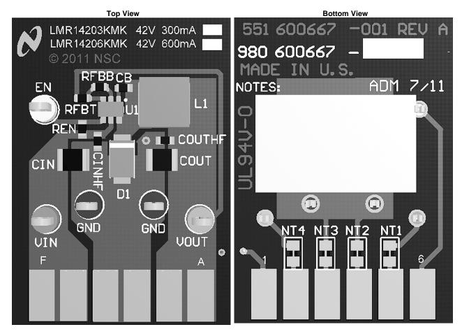
Figure 1. LMR14203/LMR14206 Demonstration Board
