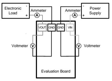
**Figure 4. Efficiency Measurements**
