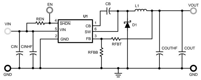
Figure 3. LMR14206 Demonstration Board Schematic
