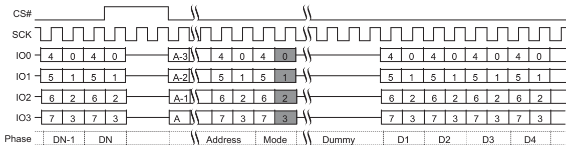
Figure 82. Continuous Quad I/O Read Command Sequence (EBh or ECh) [58, 59]
