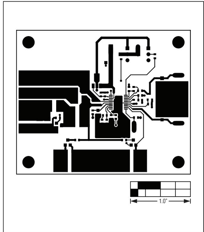
Figure 3. MAX16928 EV Kit PCB Layout—Component Side
