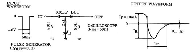
Fig.1 Reverse Recovery Time (trr) Test Circuit
