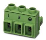
PCB connector, nominal current: 16 A, rated voltage (III/2): 400 V, number of positions: 3, pitch: 7.62 mm, connection method: Screw connection with tension sleeve, color: green, contact surface: Tin
