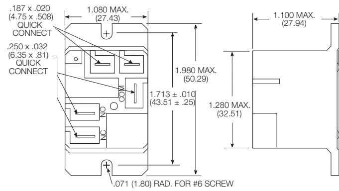
**Note:** Recommended mounting screw torque is 4.0-5.0 lbs.in when #6 screw is used.
