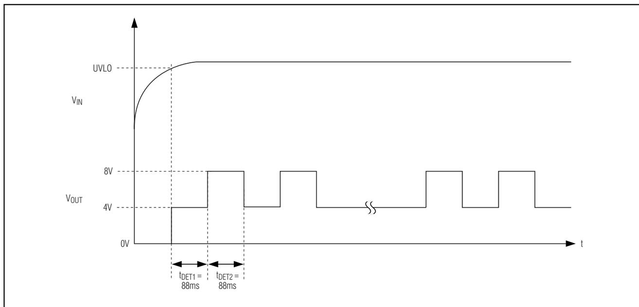
Figure 5. PD Detection with an Invalid PD Signature
