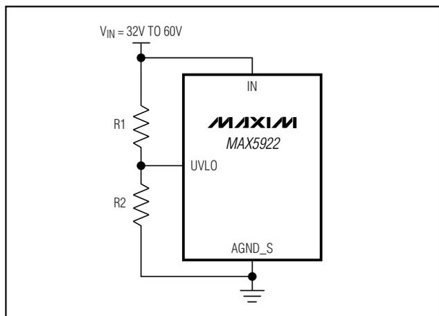
Figure 7. Setting Undervoltage Lockout with an External Resistive-Divider
