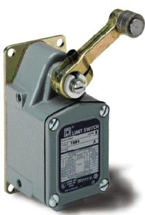
**Built for Harsh Environments.** 9007 Type T switches have extended operating and reset forces and heavy-duty contacts that will break 20A @ 120V. They also feature an ambient temperature range of up to 220° F and a die-cast zinc lever arm with hardened oil-impregnated sintered iron rollers.
