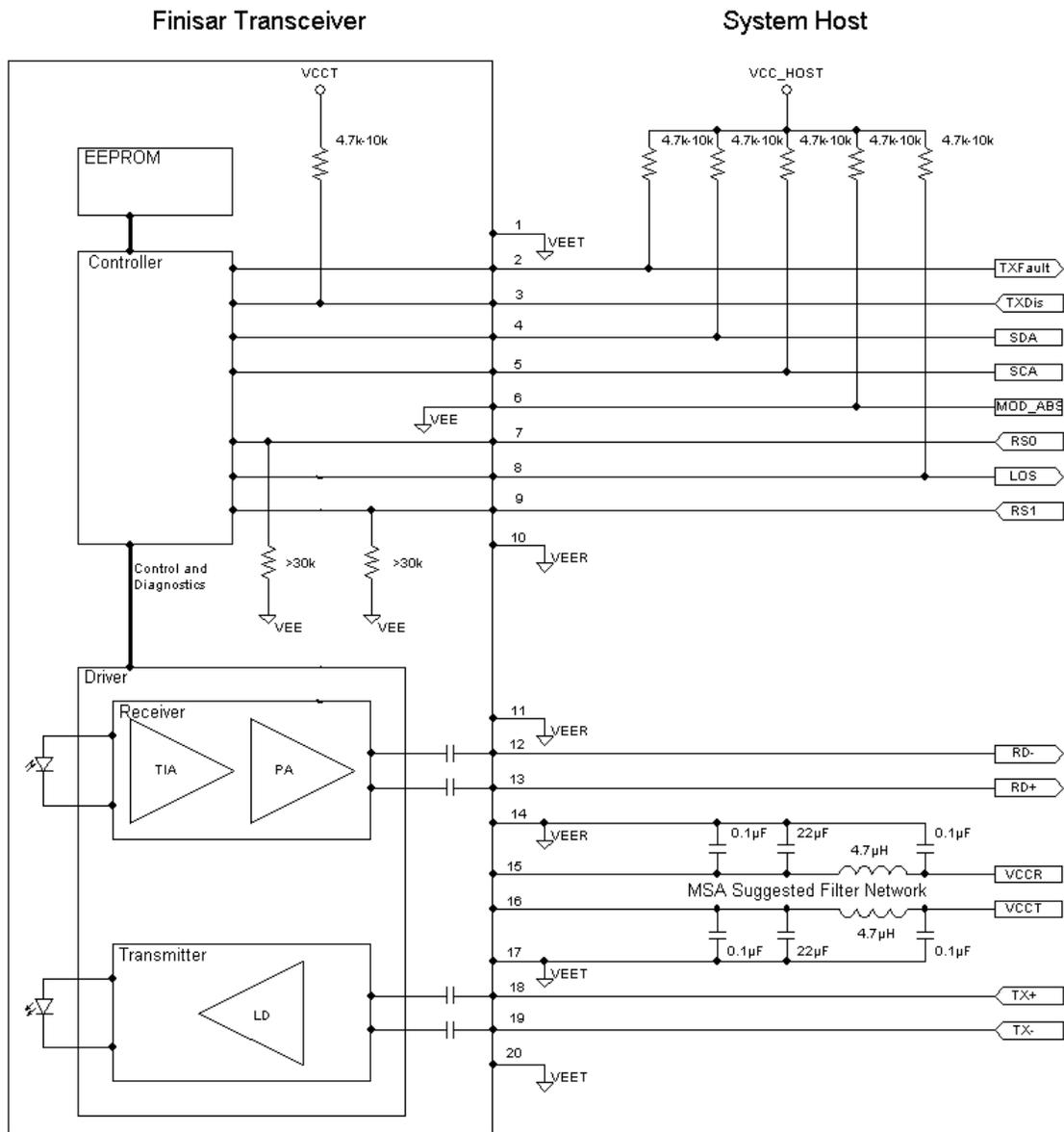
**Figure 6-Host-Module Interface**
