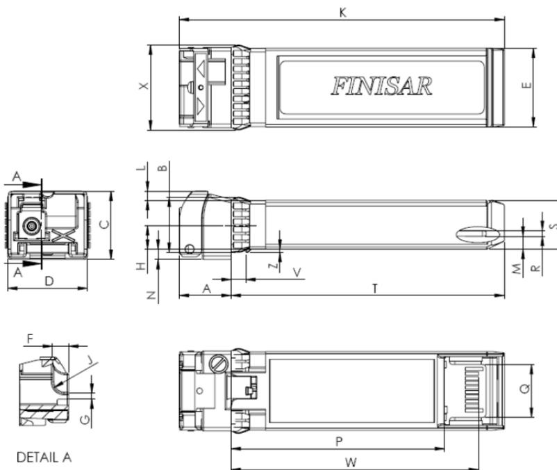
**Figure 2. FTLX2071D327/FTLX2071D333 Mechanical Dimensions**
