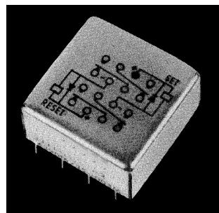
The dual coil version of the 3SBM magnetic latching relay is now available with coil transient suppression with or without blocking diodes for reverse polarity protection. This hybrid magnetic latching relay is an addition to the growing family of .150 grid relays. The diode method is employed to limit the back EMF generated when the coil circuit is opened in order to protect other circuit components such as semiconductors. The contact load
