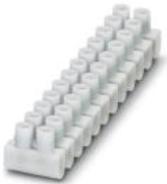
Polypropylene Europe terminal strip, white, for connecting solid conductors and stranded conductors with and without ferrules with a cross section of 0.5 to 4 mm<sup>2</sup>
