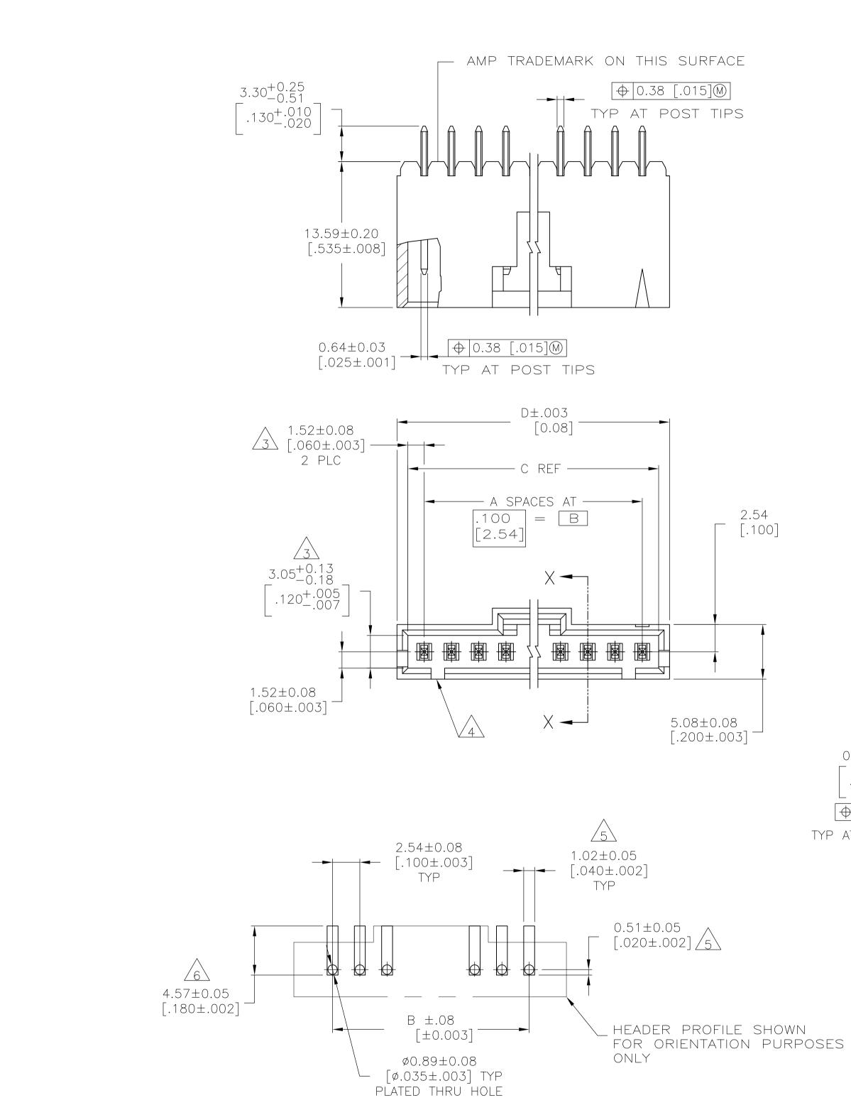
RECOMMENDED PC BOARD MOUNTING DIMENSIONS RECOMMENDED STENCIL THICKNESS = 0.25 [.010]
