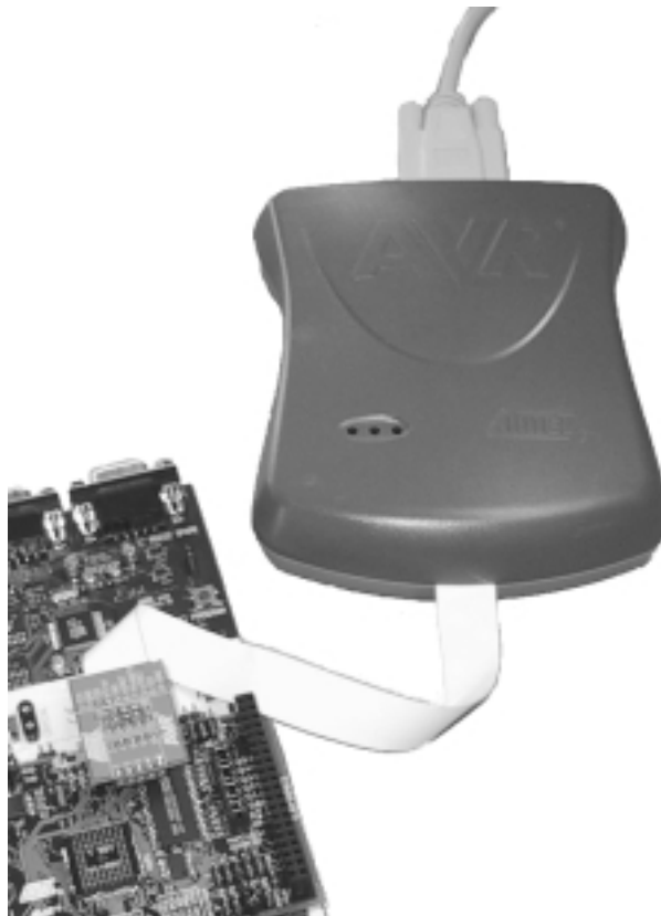
Figure 1-4. Emulating with JTAG ICE
