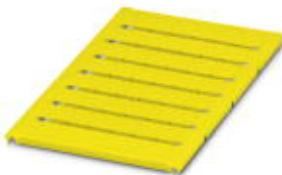
Marker for terminal blocks, Sheet, yellow, unlabeled, can be labeled with: BLUEMARK CLED, BLUEMARK LED, Plotter, Mounting type: Snap into tall marker groove, for terminal block width: 10.2 mm, Lettering field: 9.6 x 10.5 mm
