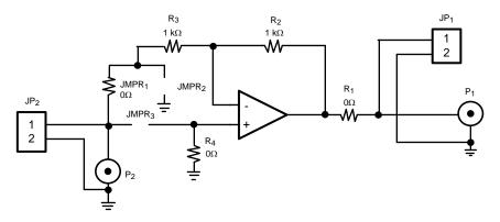
Figure 2. Inverting Amplifier
