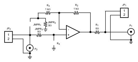
Figure 3. Non-Inverting Amplifier
