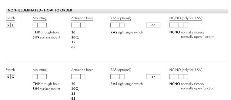
Ordering example: 5ESH935 (non-illuminated), 5GTH9658222 (illuminated), 5GSH935NCNO (normally closed/normally open); 5ETH920RAS (right angle) 5ETH920Q or 5GSH92061Q (quiet versions)
