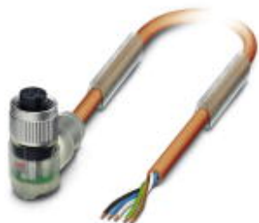
Sensor/actuator cable, 5-position, PUR halogen-free, irradiated, orange RAL 2003, free cable end, on Socket angled M12, A-coded, with 3 LEDs, cable length: 10 m, Customer-specific version
