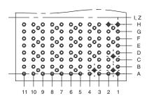
Recommended PCB hole mounting pattern for row differential applications (same geometry as above without the ground vias)
