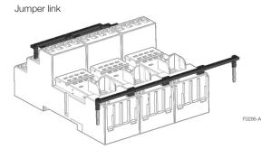
When connecting more than 2 poles with staggered jumper bars the lower bars need to be stripped and shortened to an appropriate length to enable correct fitting.
