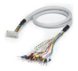
Round cable assembled with a 16-pos. socket strip and an open end. On the open end, the wires are labeled with 1 to 16 and have ferrules, cable length: 1.0 m
