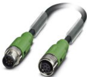
Sensor/actuator cable, 8-position, PUR halogen-free, black-gray RAL 7021, shielded, Plug straight M12 SPEEDCON, on Plug straight M12 SPEEDCON, cable length: 3 m
