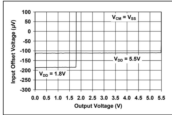
**FIGURE 2-11:** Input Offset Voltage vs. Output Voltage.
