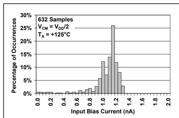
**FIGURE 2-6:** Input Bias Current at  $+125^\circ\text{C}$ .
