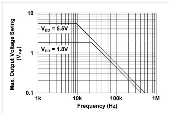
**FIGURE 2-15:** Maximum Output Voltage Swing vs. Frequency.
