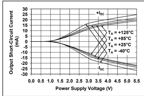
**FIGURE 2-12:** Output Short-Circuit Current vs. Ambient Temperature.
