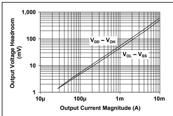
**FIGURE 2-14:** Output Voltage Headroom vs. Output Current Magnitude.
