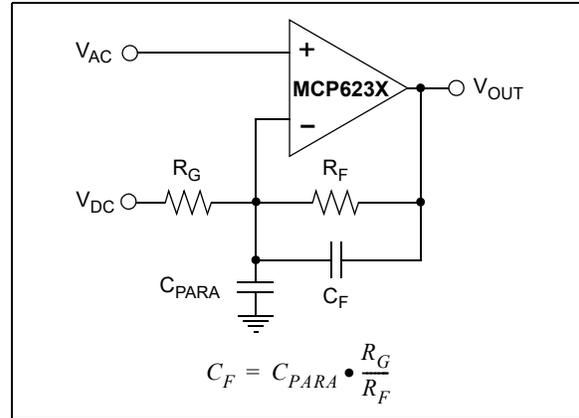
**FIGURE 4-9:** Effect of Parasitic Capacitance at the Input.
