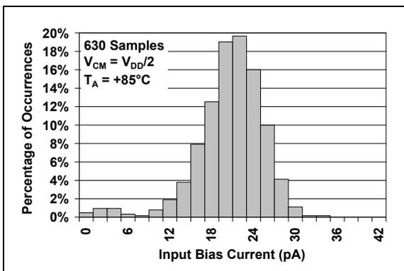
**FIGURE 2-3:** Input Bias Current at  $+85^\circ\text{C}$ .
