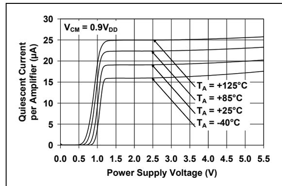
**FIGURE 2-18:** Quiescent Current vs. Power Supply Voltage.
