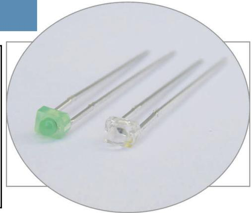
Bivar 1.8mm Package 2 mA Low Current LED is special binned at 2 mA and is ideal for those applications where lower power budget and smaller indication lighting are required such as solar panel or battery-powered portable devices. Bivar offers water clear LED lens for maximum light output and diffused LED lens for uniform light output, The Shouldered Lead frame LED has a built in strain relief feature which is ideal for Right Angle Holder assemblies that require lead bends.
