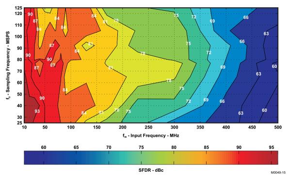
Figure 88. SFDR Contour (no gain,  $F_s = 2 V_{PP}$ )
