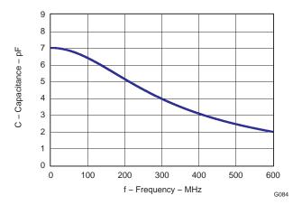
Figure 95. ADC Input Capacitance, Cin
