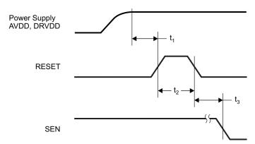
NOTE: A high-going pulse on the RESET pin is required in serial interface mode in the case of initialization through a hardware reset. For parallel interface operation, RESET has to be tied permanently HIGH.
