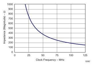
Figure 101. Clock Buffer Input Impedance
