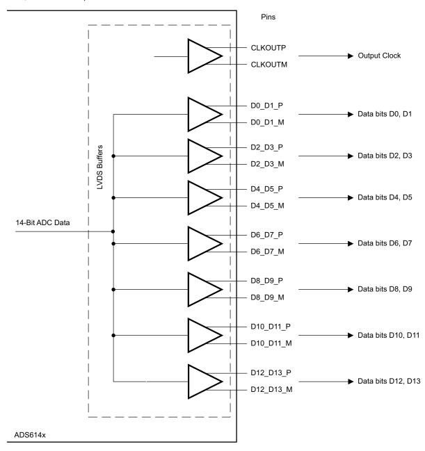
Figure 105. DDR LVDS Outputs
