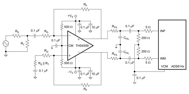
Figure 98. Drive Circuit Using the THS4509
