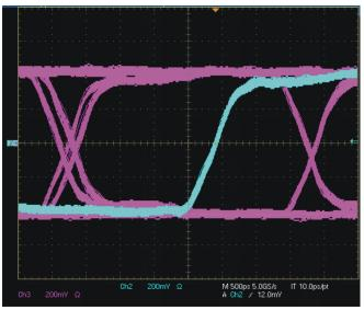
Figure 107. LVDS Eye Diagram - No Internal Termination 5-pF Load Capacitance
