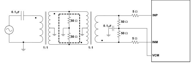
Figure 97. Two Transformer Drive Circuit
