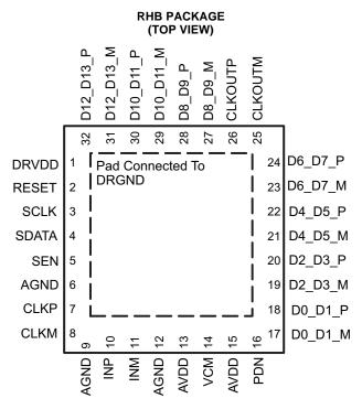
Figure 8. LVDS Mode Pinout
