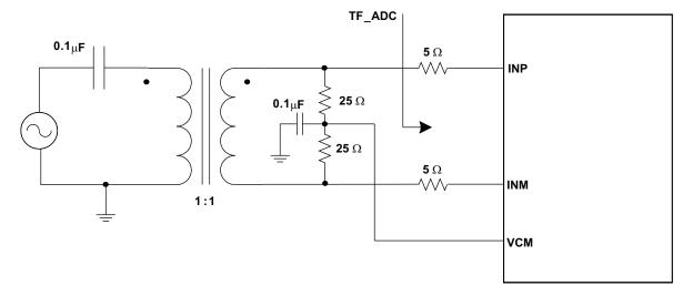
Figure 96. Single Transformer Drive Circuit
