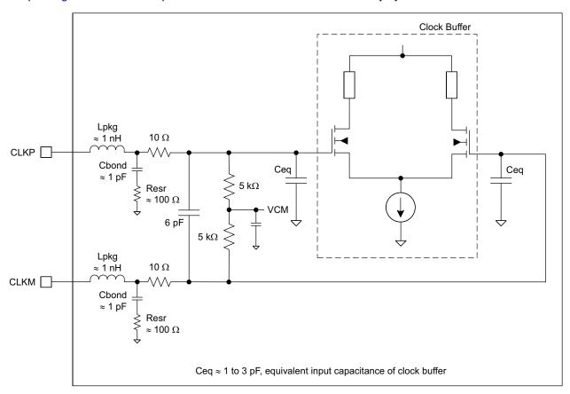
Figure 100. Internal Clock Buffer
