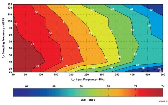
Figure 91. SNR Contour (with 3.5 dB coarse gain,  $F_S = 1.34 V_{PP}$ )
