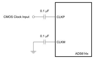
Figure 103. Single-Ended Clock Driving Circuit
