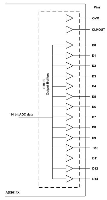
Figure 104. CMOS Output Buffers
