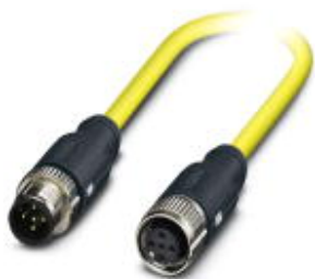
Sensor/actuator cable, 5-position, PVC, yellow, shielded, Plug straight M12 SPEEDCON, coding: A, on Socket straight M12 SPEEDCON, coding: A, cable length: 0.5 m
