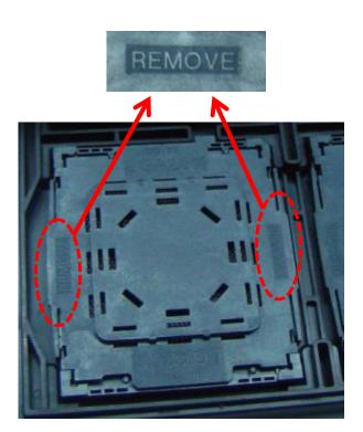
Pick up the sockets on the remove latch with two fingers
