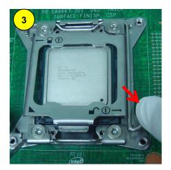
Disengage the lever slowly with one hand while holding the load plate with other hand (finger)
