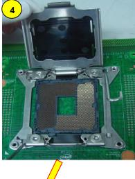
WARNING: High risk of bent pins, don't touch terminal side Install Processor Before Removing Cover.
