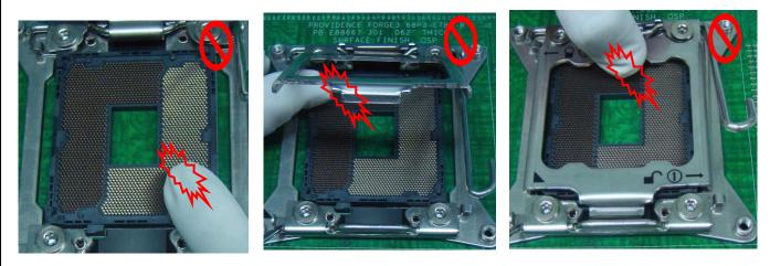
\* Don't touch the terminal side when assembled, inspection.ect. Save and replace the ILM cover when Package removed.
