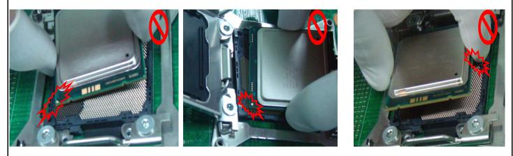
\* Use vertical motion only during package insertion / removal.
