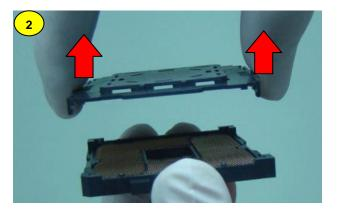
\* It is not recommended to install or remove the PnP cover before the socket solder to PCB. Don't
