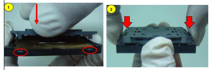
\* It is not recommended to install or remove the PnP cover before the socket solder to PCB. Don't
