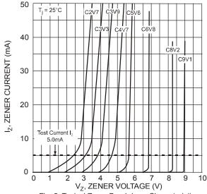
Fig. 2 Typical Zener Breakdown Characteristics
