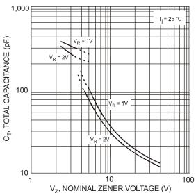
Fig. 5 Typical Total Capacitance vs. Nominal Zener Voltage
