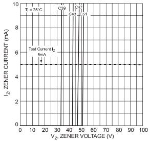
Fig. 4 Typical Zener Breakdown Characteristics
