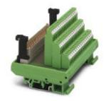
VARIOFACE module, for IEC 603/DIN 41612 connector, type F, 48-pos., z, b, d components mounted, with male connector, cable housing with latch interlock
