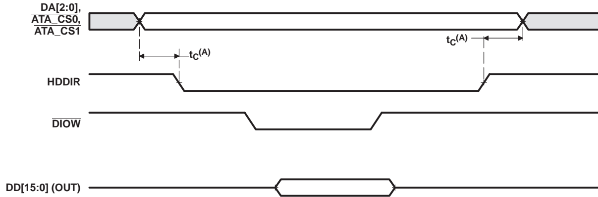
Figure 6-38. ATA/CF HDDIR Taskfile Write/Single PIO Write Timing
