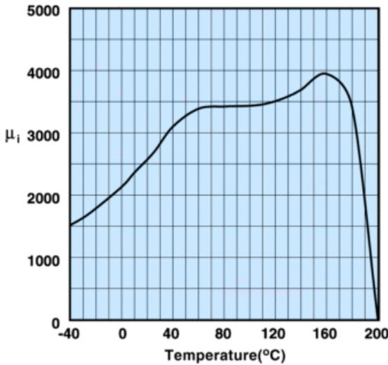
Measured on a 17/10/6mm toroid at 10kHz.
