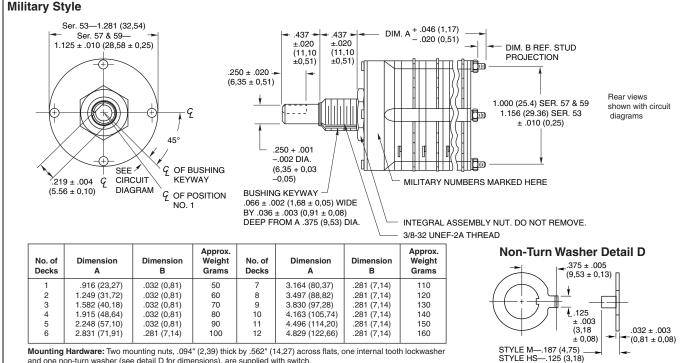
and one non-turn washer (see detail D for dimensions), are supplied with switch
