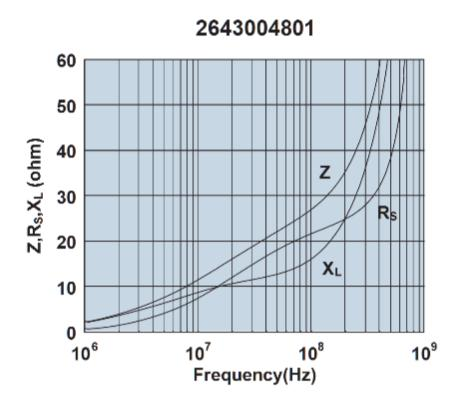
Impedance, reactance, and resistance vs. frequency.
