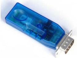
• Slave Mode- Bluetooth clients, such as Palm/Pocket PC PDA's, laptops, scanners, cellphones directly connect to FireFly via Bluetooth Serial Port Profile, creating a Virtual COM port on the client.
