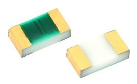
The terminations consist of an adhesion layer, a leach resistant nickel barrier and gold plating compatible with high temperature solder systems.
