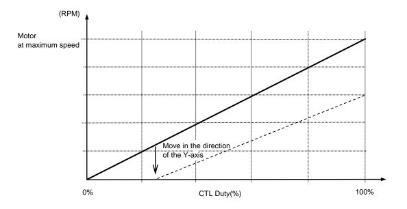
(Example) In the case where the characteristics change from ones with the origin point (0%, 0 rpm) to ones where the speed at a duty ratio of 25% becomes 0 rpm:
