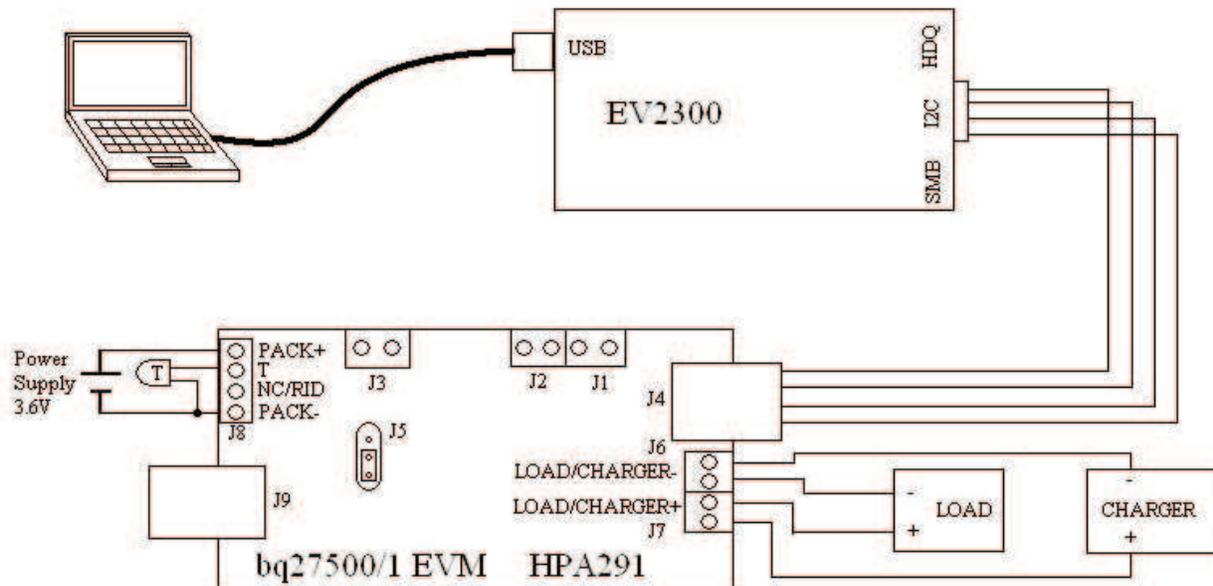
Figure 6. bq27500 Circuit Module Connection to Cell and System Load/Charger
