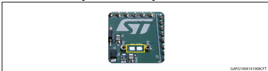
Figure 5: Pads for soldering SMD resistor
