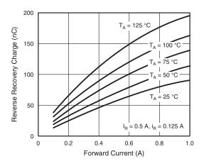
Fig. 6 - Max. Reverse Recovery Charge vs. Forward Current
