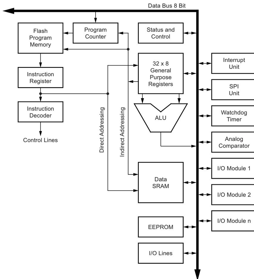
In order to maximize performance and parallelism, the Atmel AVR<sup>®</sup> uses a harvard architecture – with separate memories and buses for program and data. Instructions in the program memory are executed with a single level pipelining. While one instruction is being executed, the next instruction is pre-fetched from the program memory. This concept enables instructions to be executed in every clock cycle. The program memory is in-system reprogrammable flash memory.
