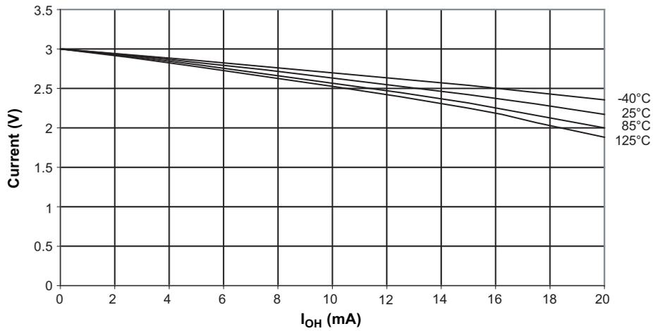
Figure 6-13. Reset Pull-Up Resistor Current versus Reset Pin Voltage ( $V_{CC} = 5V$ )
