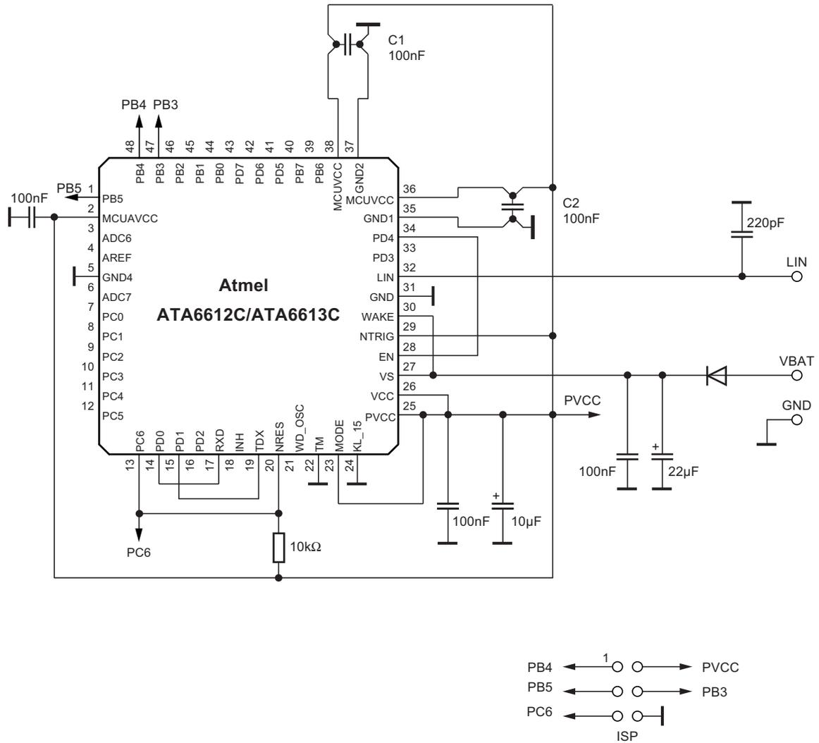
Note: All open pins of the SiP can be used for application-specific purposes.
