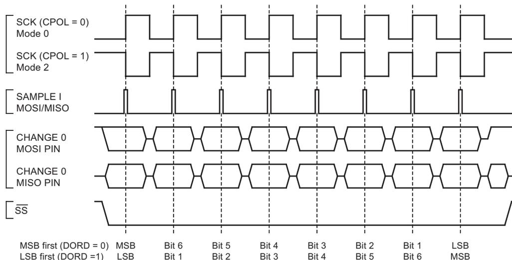
**Figure 5-68. SPI Transfer Format with CPHA = 1**
