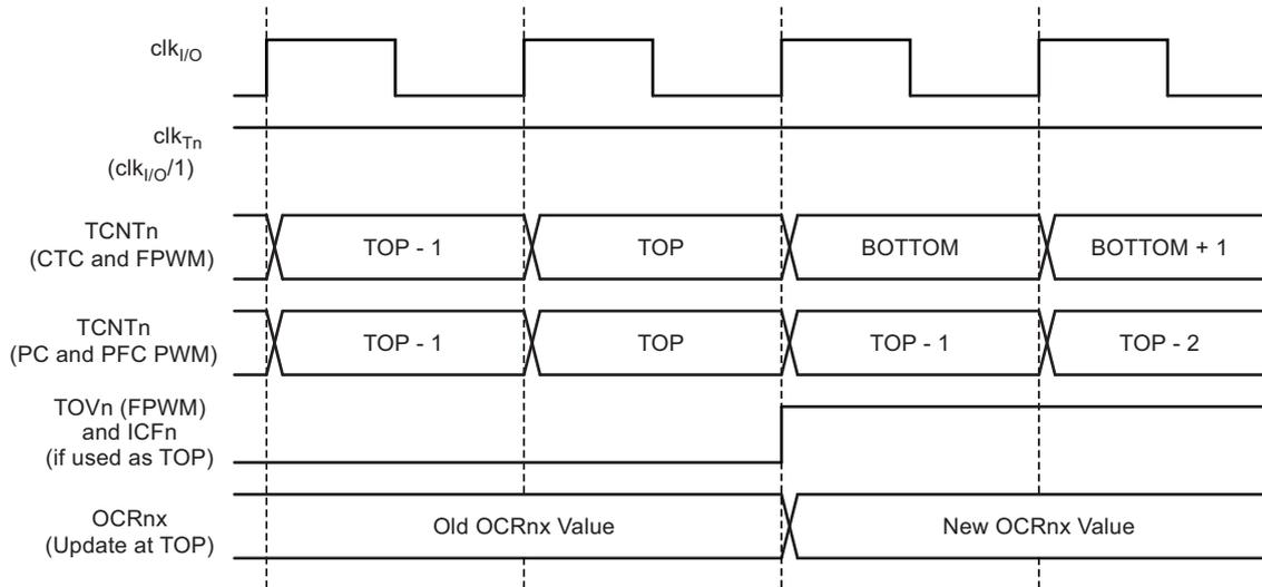
Figure 5-52 shows the same timing data, but with the prescaler enabled.
