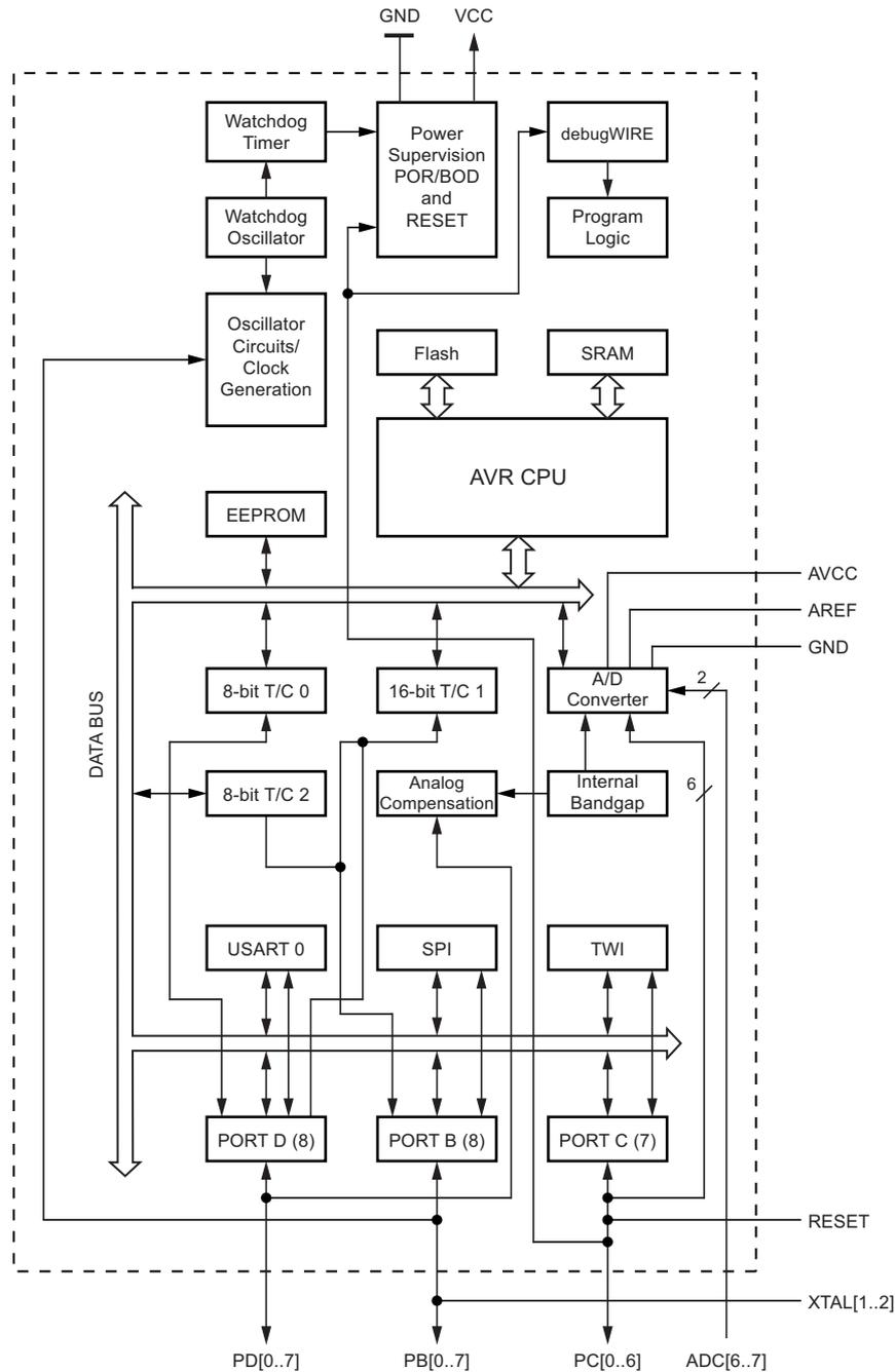
The Atmel® AVR® core combines a rich instruction set with 32 general purpose working registers. All the 32 registers are directly connected to the arithmetic logic unit (ALU), allowing two independent registers to be accessed in one single instruction executed in one clock cycle. The resulting architecture is more code efficient while achieving throughputs up to ten times faster than conventional CISC microcontrollers.
