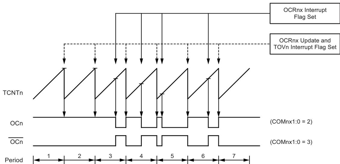
The Timer/Counter overflow flag (TOV2) is set each time the counter reaches TOP. If the interrupt is enabled, the interrupt handler routine can be used for updating the compare value.
