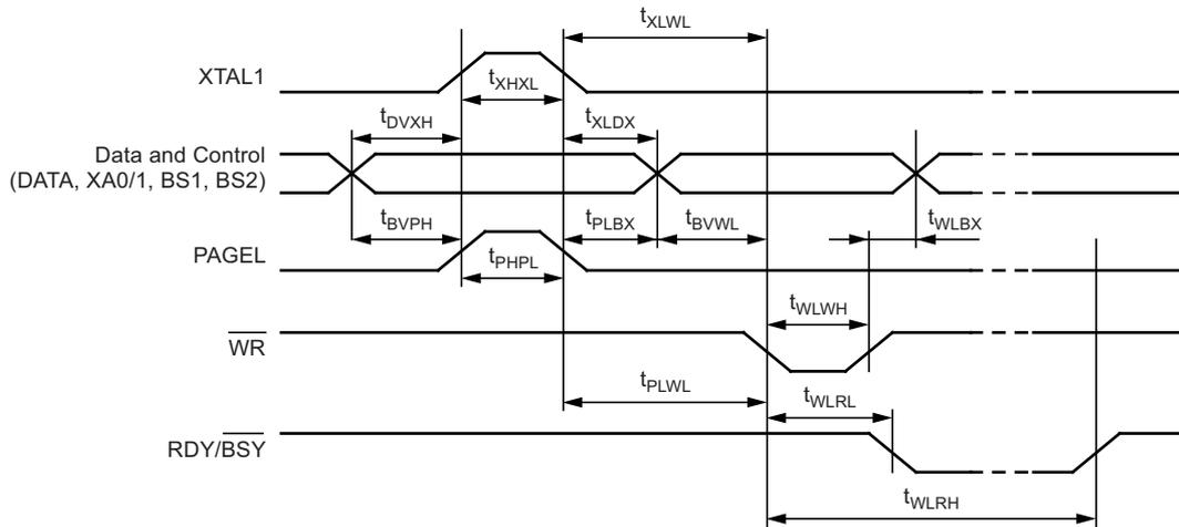
**Figure 5-124. Parallel Programming Timing, Loading Sequence with Timing Requirements<sup>(1)</sup>**
