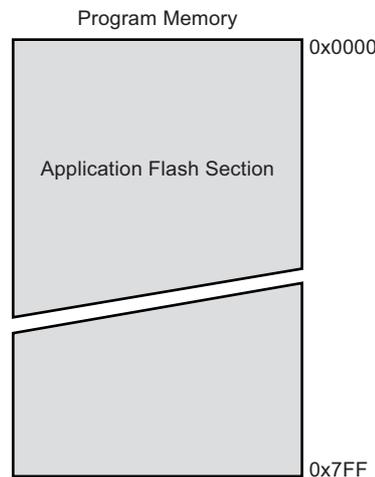
**Figure 5-8. Program Memory Map, Atmel ATA6612C/ATA6613C**
