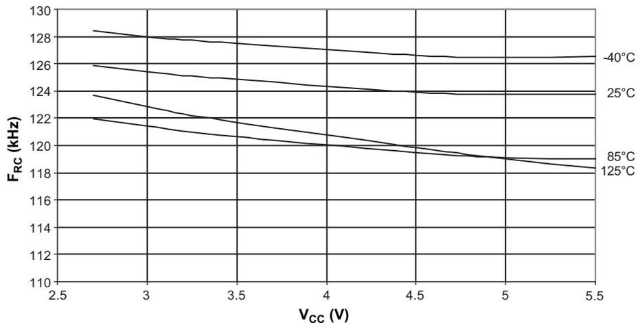
Figure 6-23. Calibrated 8MHz RC Oscillator Frequency versus Temperature
