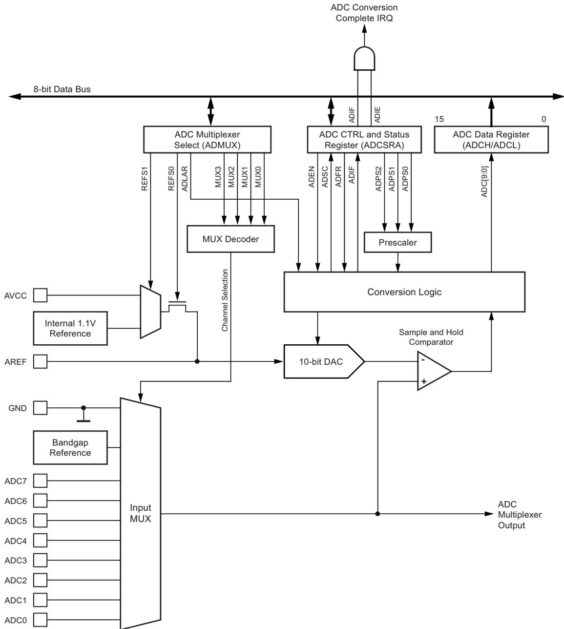
The ADC converts an analog input voltage to a 10-bit digital value through successive approximation. The minimum value represents GND and the maximum value represents the voltage on the AREF pin minus 1LSB. Optionally,  $AV_{CC}$  or an internal 1.1V reference voltage may be connected to the AREF pin by writing to the REFSn bits in the ADMUX register. The internal voltage reference may thus be decoupled by an external capacitor at the AREF pin to improve noise immunity.
