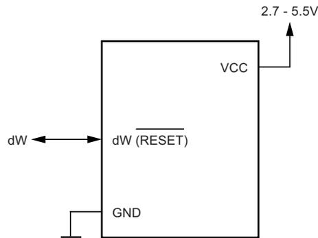
Figure 5-113 shows the schematic of a target MCU, with debugWIRE enabled, and the emulator connector. The system clock is not affected by debugWIRE and will always be the clock source selected by the CKSEL fuses.
