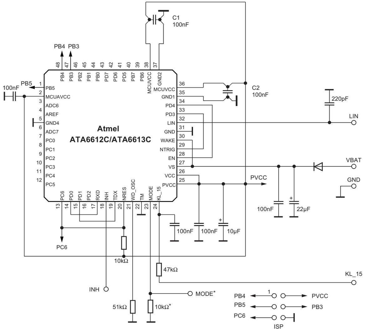
\* The MODE pin can be connected directly to GND, if it is not needed to disable the Watchdog
