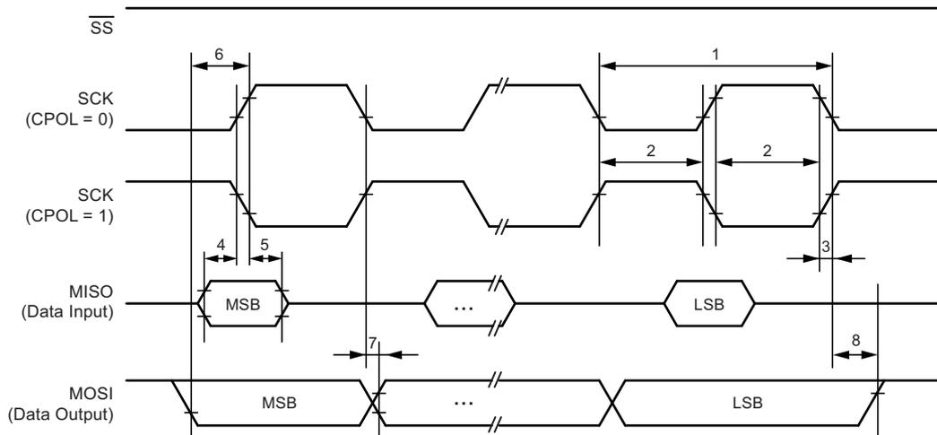
**Figure 6-3. SPI Interface Timing Requirements (Slave Mode)**
