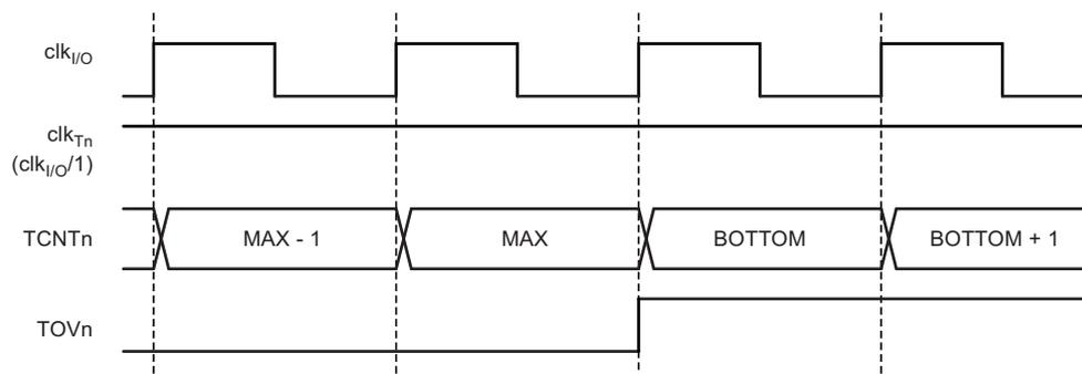
Figure 5-61 shows the same timing data, but with the prescaler enabled.
