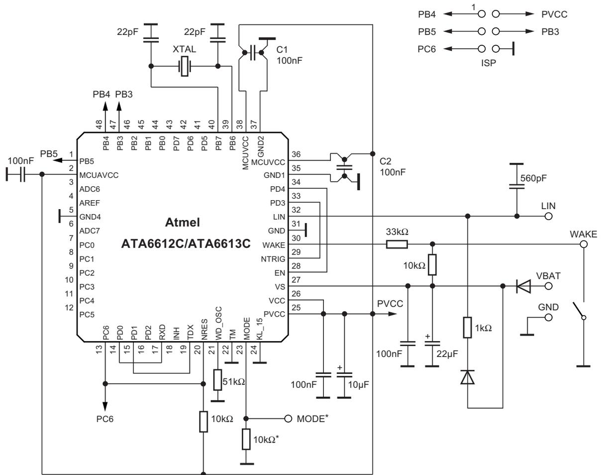
\* The MODE pin can be connected directly to GND, if it is not needed to disable the Watchdog
