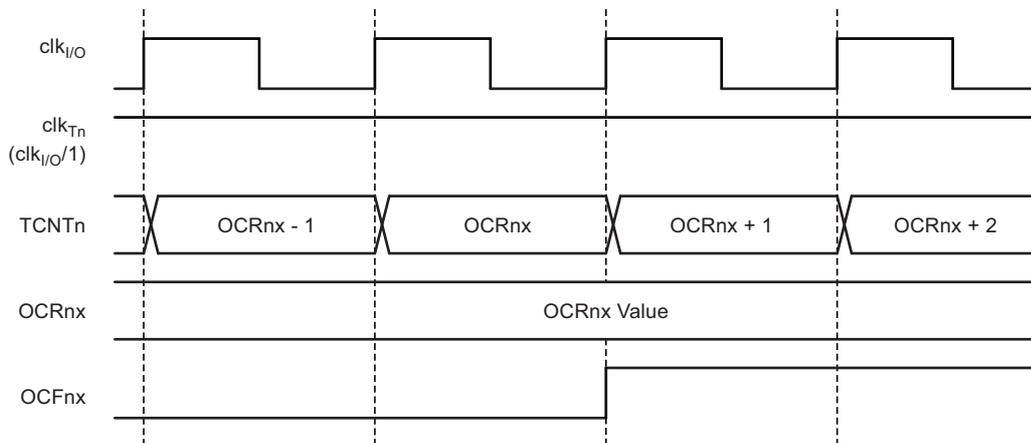
[Figure 5-50](#) shows the same timing data, but with the prescaler enabled.
