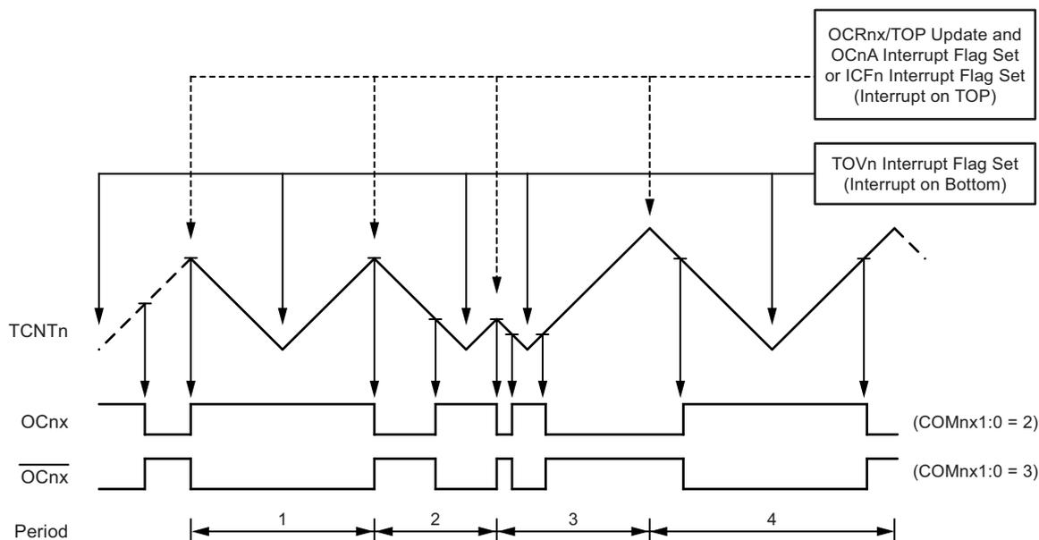
The Timer/Counter overflow flag (TOV1) is set each time the counter reaches BOTTOM. When either OCR1A or ICR1 is used for defining the TOP value, the OC1A or ICF1 flag is set accordingly at the same timer clock cycle as the OCR1x registers are updated with the double buffer value (at TOP). The interrupt flags can be used to generate an interrupt each time the counter reaches the TOP or BOTTOM value.
