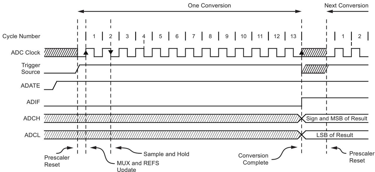
**Figure 5-106. ADC Timing Diagram, Free Running Conversion**
