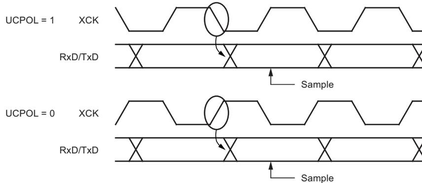
The UCPOLn bit UCRSC selects which XCKn clock edge is used for data sampling and which is used for data change. As Figure 5-71 shows, when UCPOLn is zero the data will be changed at rising XCKn edge and sampled at falling XCKn edge. If UCPOLn is set, the data will be changed at falling XCKn edge and sampled at rising XCKn edge.
