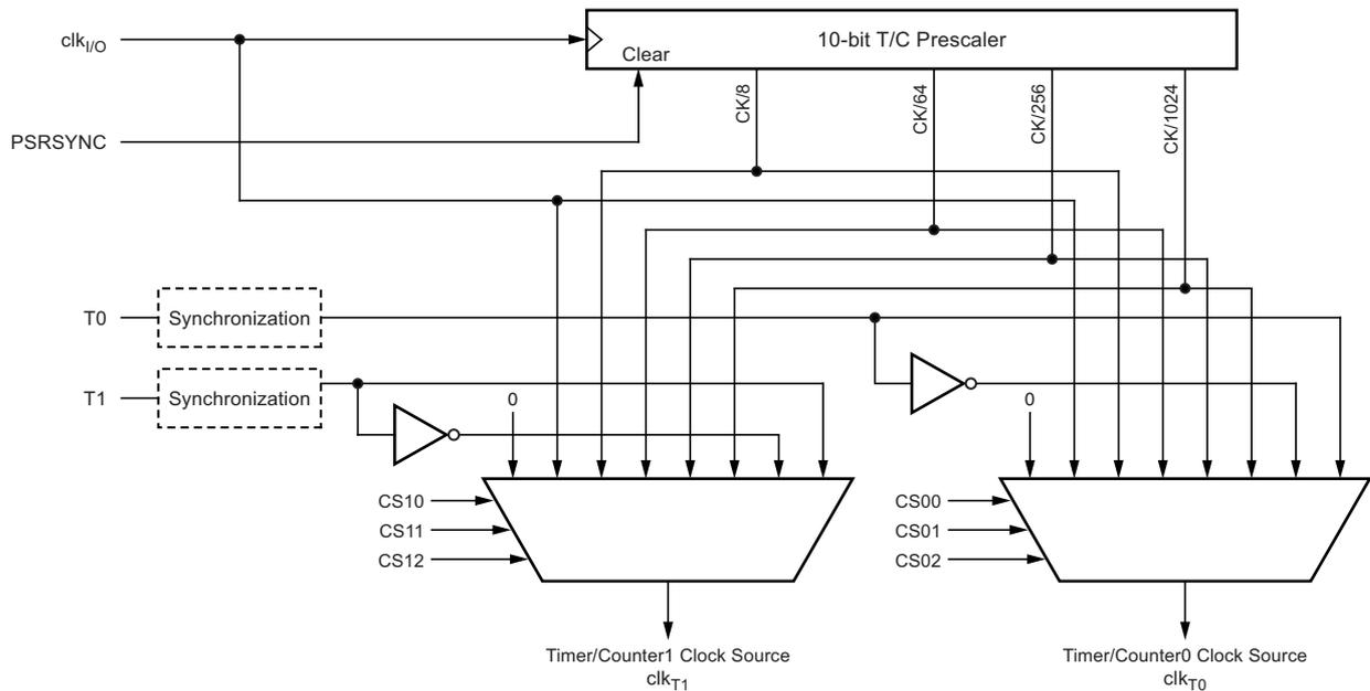
Note: 1. The synchronization logic on the input pins (T1/T0) is shown in [Figure 5-38 on page 112](#).
