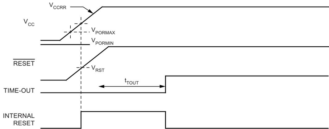
**Figure 5-17. MCU Start-up,  $\overline{\text{RESET}}$  Extended Externally**
