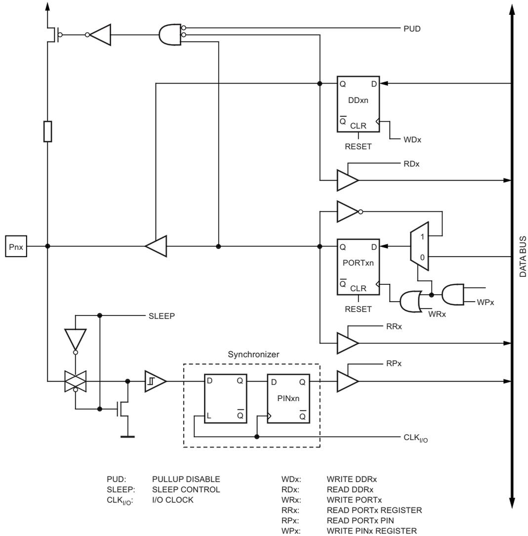
Note: 1. WRx, WPx, WDx, RRx, RPx, and RDx are common to all pins within the same port. clk<sub>I/O</sub>, SLEEP, and PUD are common to all ports.
