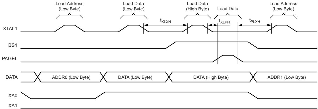
Note: 1. The timing requirements shown in [Figure 5-123 on page 265](#) (i.e.,  $t_{DVXH}$ ,  $t_{XHXL}$ , and  $t_{XLDX}$ ) also apply to loading operation.
