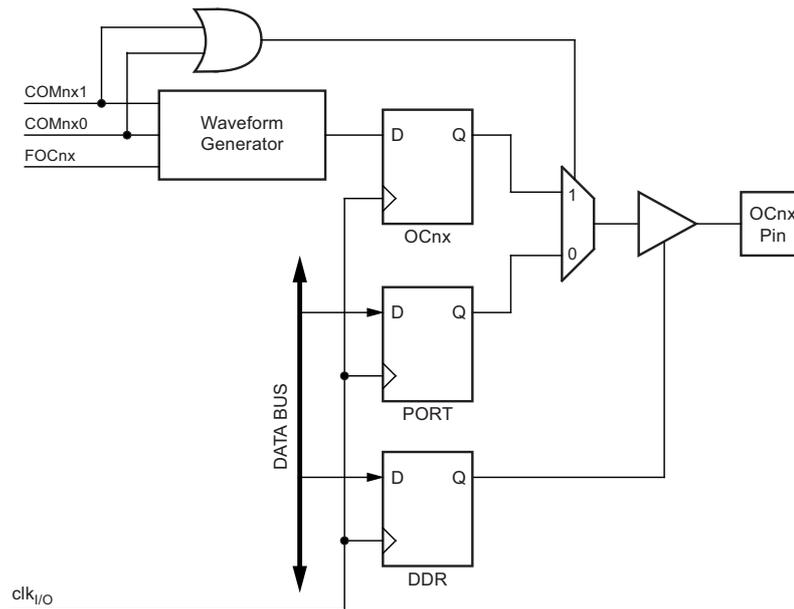
The general I/O port function is overridden by the output compare (OC0x) from the waveform generator if either of the COM0x1:0 bits are set. However, the OC0x pin direction (input or output) is still controlled by the data direction register (DDR) for the port pin. The data direction register bit for the OC0x pin (DDR\_OC0x) must be set as output before the OC0x value is visible on the pin. The port override function is independent of the waveform generation mode.
