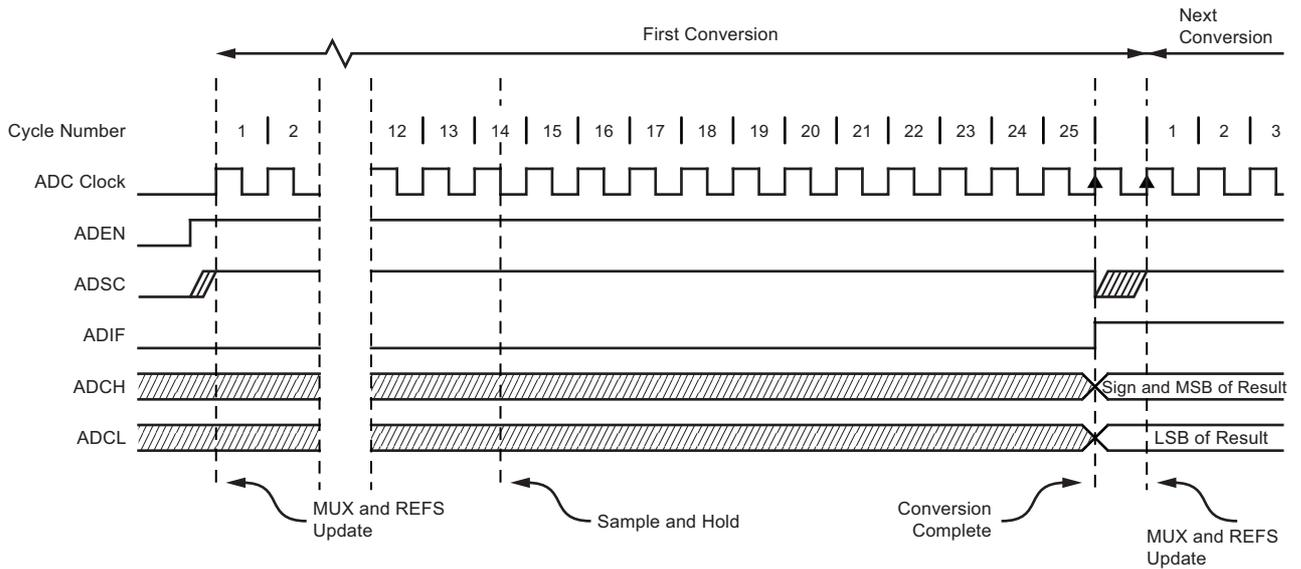
**Figure 5-104. ADC Timing Diagram, Single Conversion**
