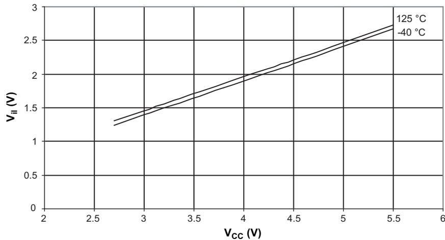
**Figure 6-20. Reset Input Threshold Voltage versus  $V_{CC}$  ( $V_{IH}$ , Reset Pin Read as 1)**
