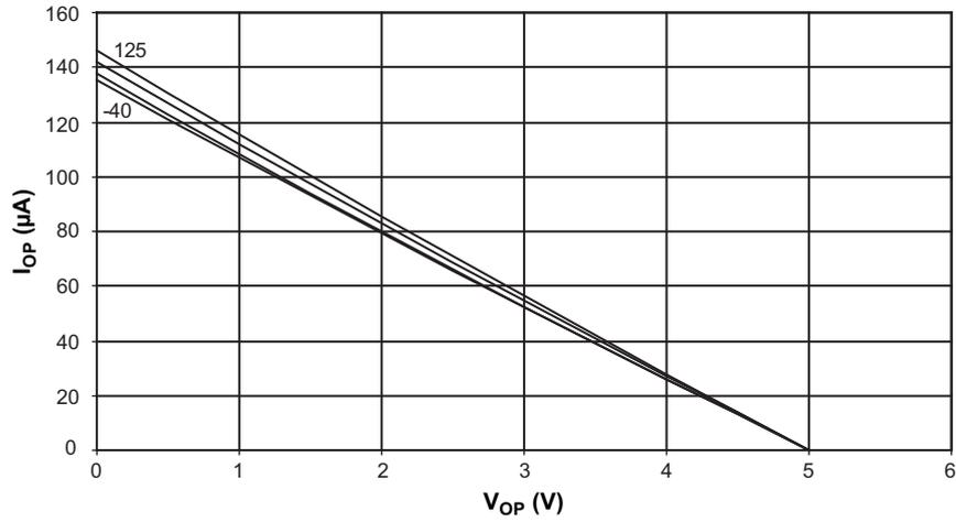
Figure 6-9. Output Low Voltage versus Output Low Current ( $V_{CC} = 5V$ )
