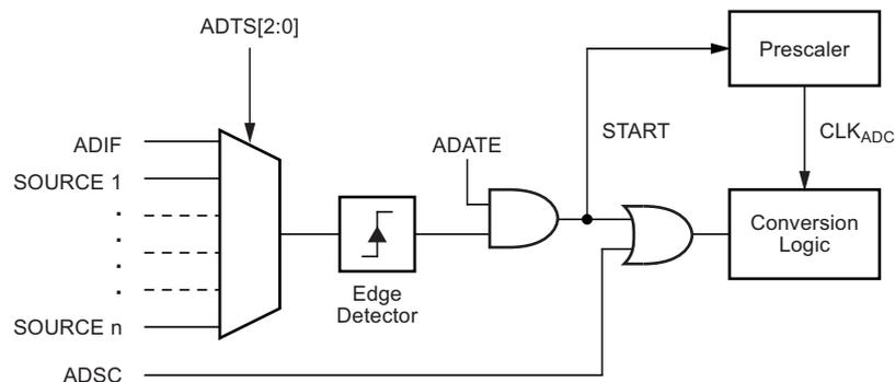
Using the ADC interrupt flag as a trigger source makes the ADC start a new conversion as soon as the ongoing conversion has finished. The ADC then operates in free running mode, constantly sampling and updating the ADC data register. The first conversion must be started by writing a logical one to the ADSC bit in ADCSRA. In this mode the ADC will perform successive conversions independently of whether the ADC interrupt flag, ADIF is cleared or not.
