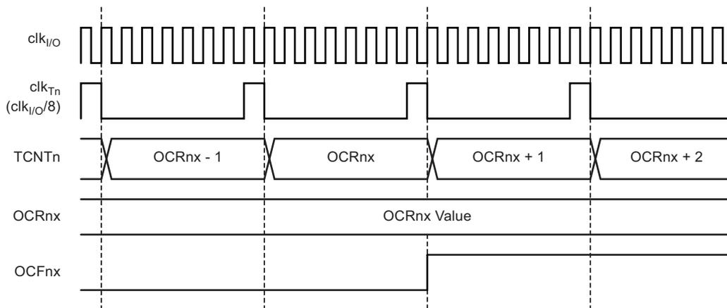
Figure 5-51 shows the count sequence close to TOP in various modes. When using phase and frequency correct PWM mode the OCR1x register is updated at BOTTOM. The timing diagrams will be the same, but TOP should be replaced by BOTTOM, TOP-1 by BOTTOM+1 and so on. The same renaming applies for modes that set the TOV1 flag at BOTTOM.
