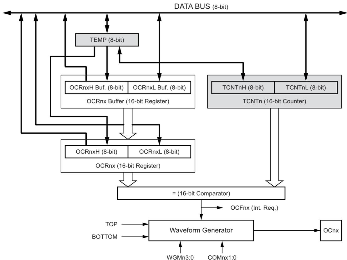
The OCR1x register is double buffered when using any of the twelve pulse width modulation (PWM) modes. For the normal and clear timer on compare (CTC) modes of operation, the double buffering is disabled. The double buffering synchronizes the update of the OCR1x compare register to either TOP or BOTTOM of the counting sequence. The synchronization prevents the occurrence of odd-length, non-symmetrical PWM pulses, thereby making the output glitch-free.
