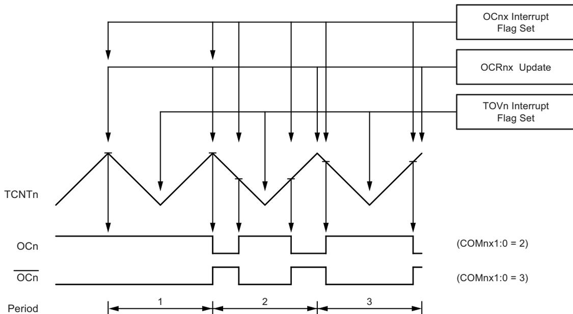
The Timer/Counter overflow flag (TOV0) is set each time the counter reaches BOTTOM. The interrupt flag can be used to generate an interrupt each time the counter reaches the BOTTOM value.
