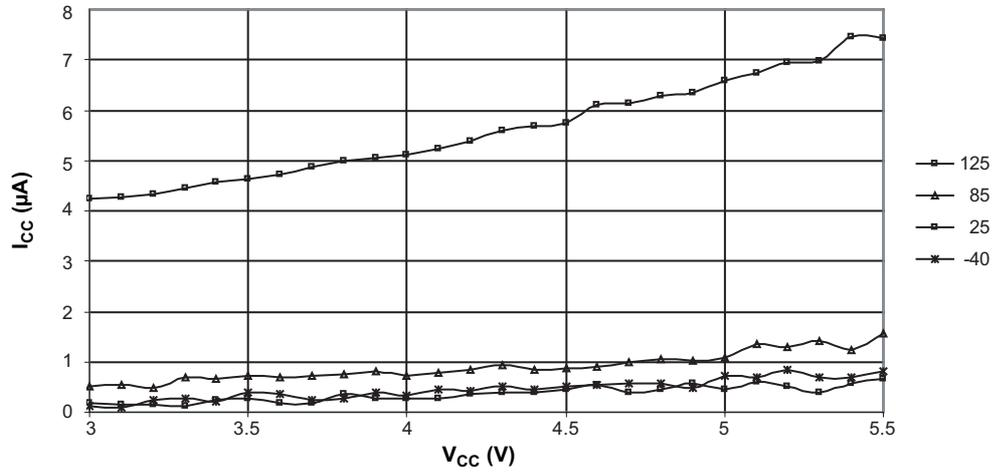
Figure 6-7. Power-down Supply Current versus  $V_{CC}$  (Watchdog Timer Enabled)
