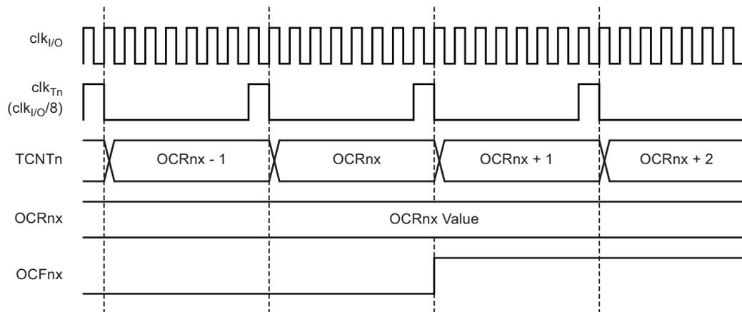
Figure 5-37 shows the setting of OCF0A and the clearing of TCNT0 in CTC mode and fast PWM mode where OCR0A is TOP.
