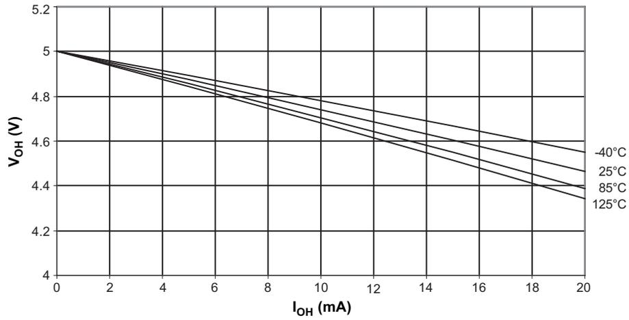
Figure 6-12. Output High Voltage versus Output High Current ( $V_{CC} = 3V$ )
