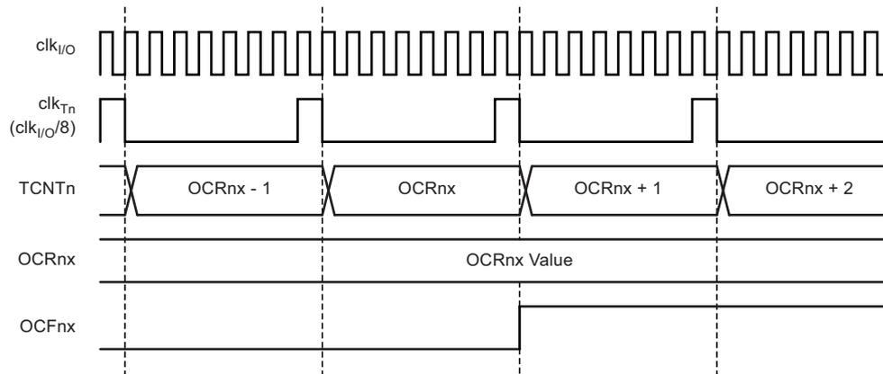
Figure 5-63 shows the setting of OCF2A and the clearing of TCNT2 in CTC mode.
