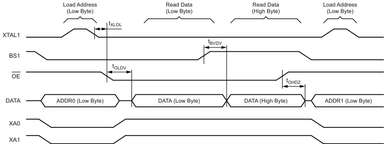
Note: 1. The timing requirements shown in [Figure 5-123 on page 265](#) (i.e.,  $t_{DVXH}$ ,  $t_{XHXL}$ , and  $t_{XLDX}$ ) also apply to reading operation.
