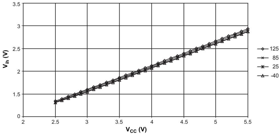
Figure 6-19. I/O Pin Input Threshold versus  $V_{CC}$  ( $V_{IL}$ , I/O Pin Read as 0)
