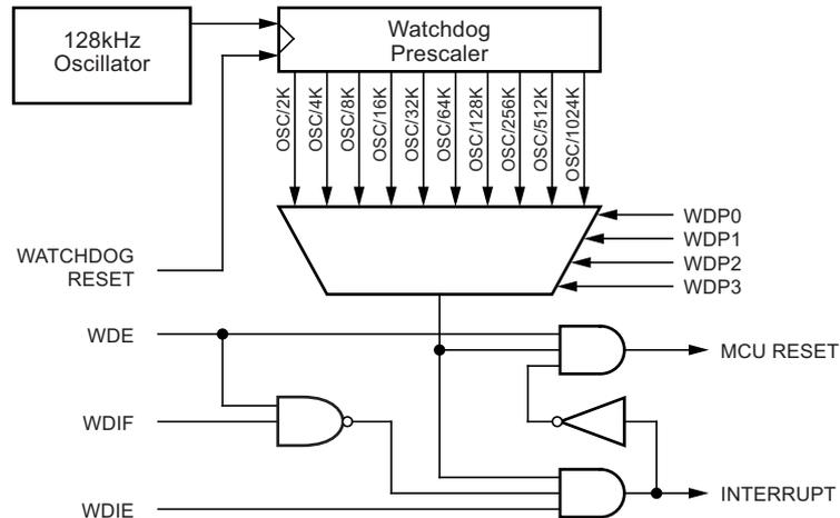
The watchdog timer (WDT) is a timer counting cycles of a separate on-chip 128kHz oscillator. The WDT gives an interrupt or a system reset when the counter reaches a given time-out value. In normal operation mode, it is required that the system uses the WDR - watchdog timer reset - instruction to restart the counter before the time-out value is reached. If the system doesn't restart the counter, an interrupt or system reset will be issued.
