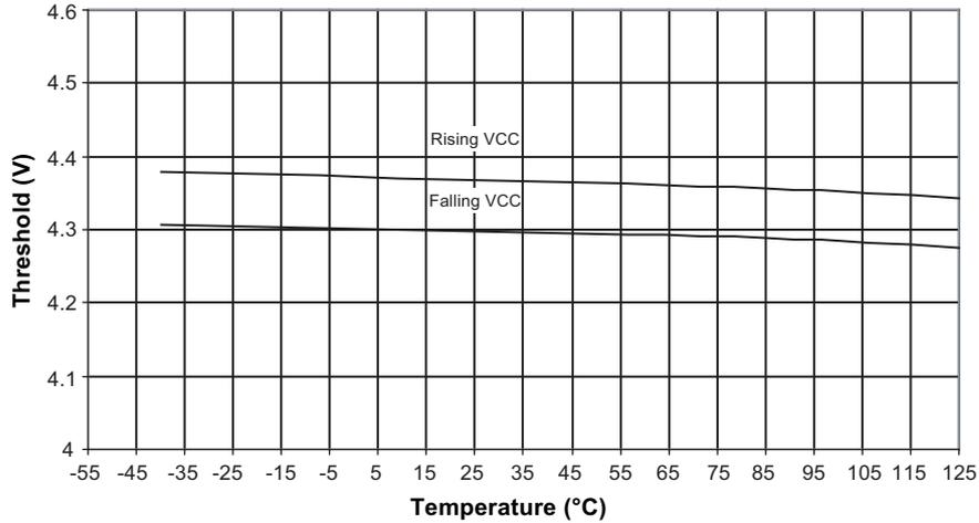
Figure 6-28. BOD Threshold versus Temperature (BODLEVEL is 2.7V)
