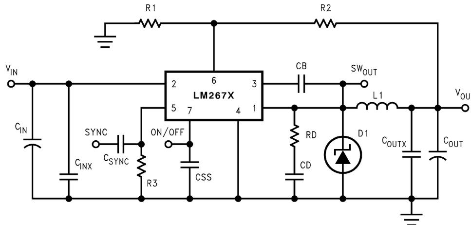
**Figure 1. Example Schematic Showing Connection for all Components.**
