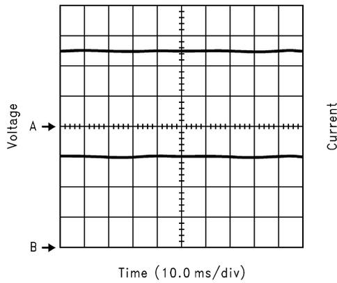
A: OUTPUT VOLTAGE:  $V_{OUT}$ ; 2V/DIV
