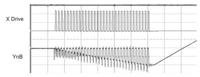
Unlike other QT circuits, the Cs capacitor values on QT1244 have no effect on conversion gain. However, they do affect conversion time.
