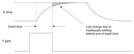
Dwell time problems can also be solved by either reducing the stray capacitance on the X line(s) (by a layout change, for example by reducing X line exposure to nearby ground planes or traces), or, the Rx resistor needs to be reduced in value (or a combination of both approaches).
