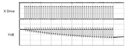
This phenomenon is more subtle. It can be best detected by increasing BL to a high count and watching what the waveform does as it descends towards and below –0.25 V. The waveform appears deceptively straight, but it slowly starts to flatten even before the –0.25 V level is reached.
