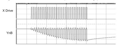
The cause of this is either from the burst length being too long, the Cs value being too small, or the X-Y transfer coupling being too large. Solutions include loosening up the key structure interleaving, greater separation of the X and Y lines on the PCB, increasing Cs, and decreasing the burst length.
