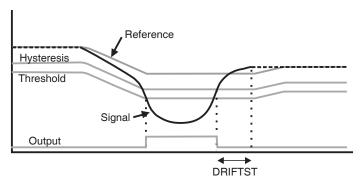
When a finger is sensed, the signal falls since the human body acts to absorb charge from the cross-coupling between X and Y lines. An isolated, untouched foreign object (a coin, or a water film) cause the signal to rise very slightly due to an enhancement of coupling. This is contrary to the way most capacitive sensors operate.
