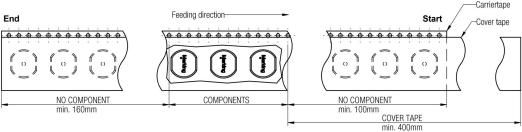
Packaging is referred to the international standard IEC 60286 -3:2007 Projection Würth Elektronik eiSos GmbH & Co. KG EMC & Inductive Solutions SSt 1.3 2014-06-26 SSt Max-Eyth-Str. 1 1.2 2014-03-26 SSt SSt 74638 Waldenburg Germany 2013-08-06 SSt SvS Tel. +49 (0) 79 42 945 - 0 Pull-of force www.we-online.com 1.0 SSt 2013-04-09 SvS Tape width | **16 mm** | 0,1 N - 1,0 N eiSos@we-online.com
