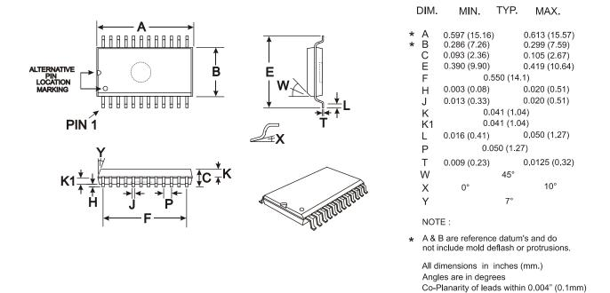
Figure 14a 24-pin SOIC (D2) Mechanical Outline: Order as part no. CMX867AD2
