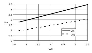
Figure 11 Typical Schmitt Trigger Input Voltage Thresholds vs. V<sub>DD</sub>
